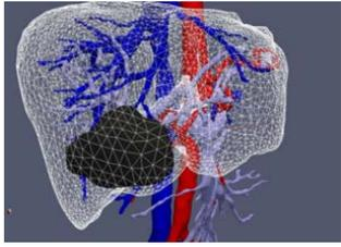
*Figure 6: 3D FEM discretization of the liver*
