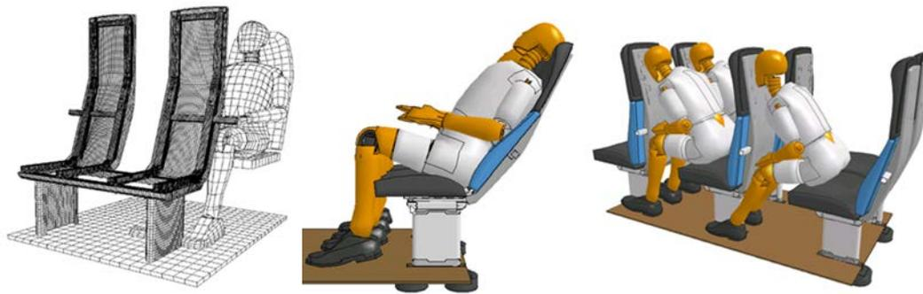
*Figure 10: Simulation of crash test of railway passenger seat.*
