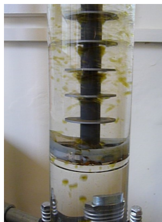
Fig: Dispersion of solvent drops by a rotating disc stack
